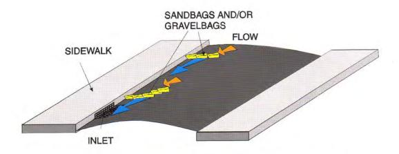
SAND OR GRAVEL BAGS (PREFERRED) USED IN ROADWAYS SERVE TO DIVERT FLOW, SLOW FLOW VELOCITY, AND POND AND FILTER RUNOFF.
