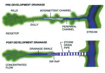
DRAINAGE PATTERNS FROM AN UNDEVELOPED VERSUS A DEVELOPED WATERSHED
